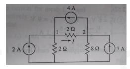
b) Determine the mesh currents  $I_1,I_2$  and  $I_3$  in the circuit given
