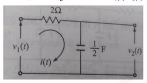
5 a) Determine the current transfer ratio  $\alpha_{12}(s)$  and transfer impedance  $Z_{21}(s)$  (8)
