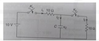
6 a) The circuit has acquired steady state with switch closed for t<0.At t=0,the switch (8) is opened .Find i(t) for t>0
